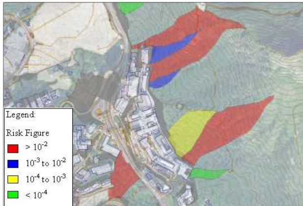
Figure 11. GIS-based landslide quantitative risk assessment
