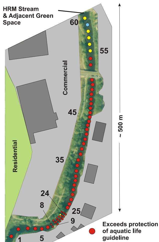
Figure 2. Schematic of HRM stream, surroundings and sampling locations (approximately 10 m apart measured along the stream axis). Numbers refer to sample stations.
