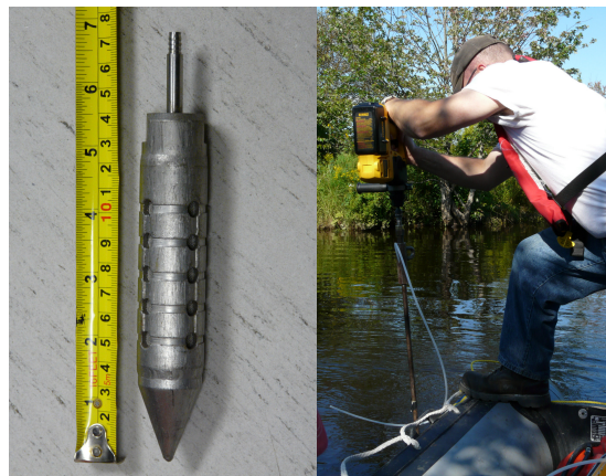
Figure 1. Sampling drive-point (left) and installation below streambed from an inflatable boat (right)
