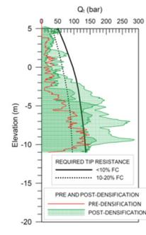
Figure 16: Effectiveness of timber compaction piles at S10
