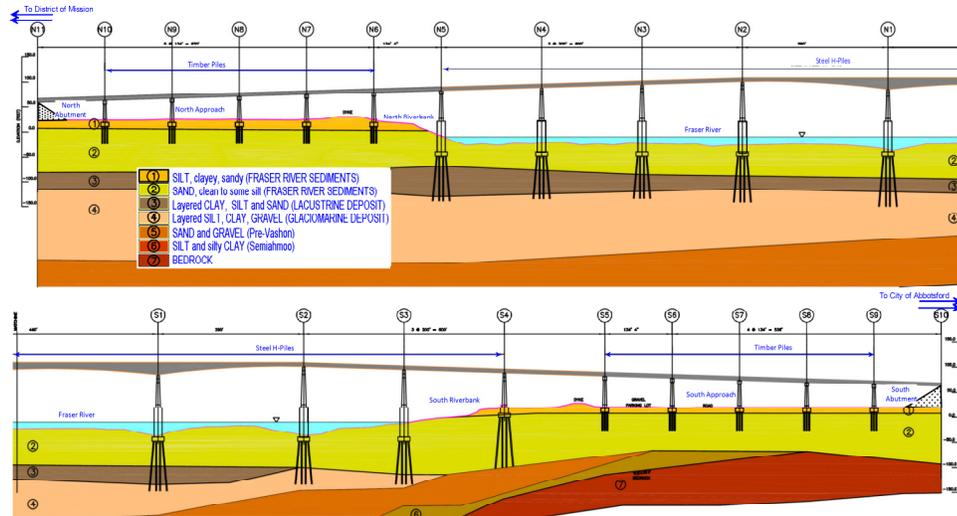
Figure 1: Geological cross-section of the Mission Bridge
