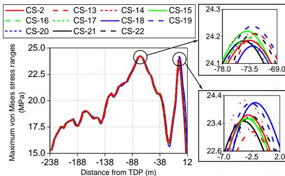
Figure 17. Effects of nonlinear soil parameters on the distribution of the maximum von Mises stress ranges along SCR on nonlinear hysteretic seabed
