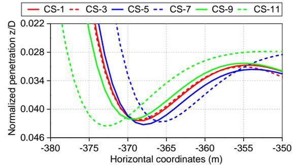
Figure 12. Final riser profiles from CS-1 to CS-11.
