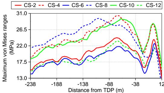
Figure 16. Effects of slug parameters on the distribution of the maximum von Mises stress ranges along SCR on nonlinear hysteretic seabed.
