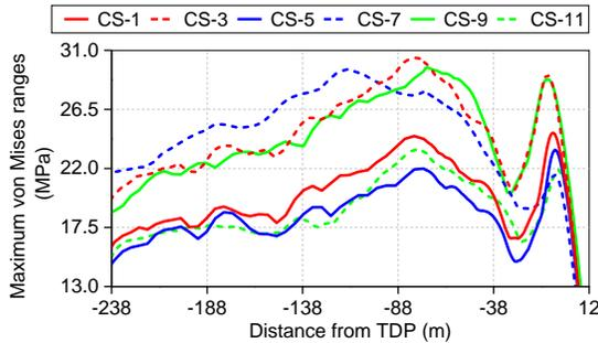
Figure 15. Effects of slug parameters on the distribution of the maximum von Mises stress ranges along SCR on elastic seabed.
