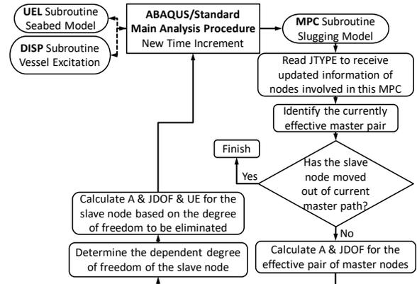
Figure 4. MPC subroutine internal flowchart.
