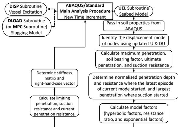
Figure 5. UEL subroutine internal flowchart.
