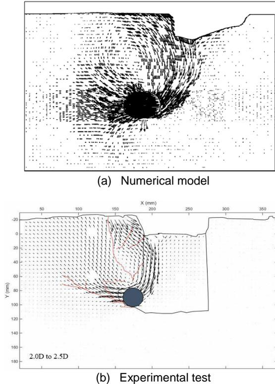
Figure 10. Vectorial displacement for pipe movement from 2.0D to 2.5D
