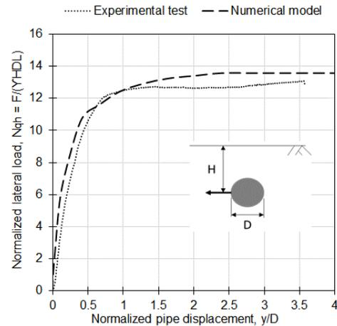
Figure 9. Normalised lateral load
