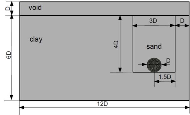
Figure 2. configuration of numerical model
