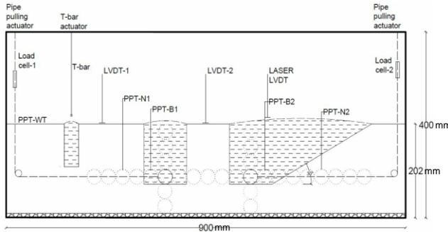
Figure 1. Configuration of experimental test
