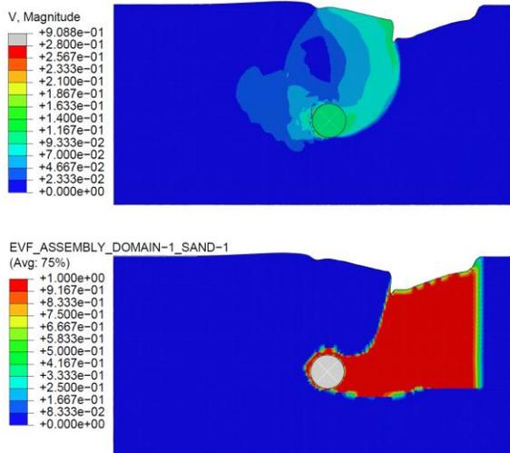
Figure 6. Pipeline laterally displaced by 2D-3D.
