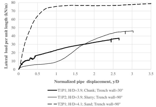
Figure 11. Effect of backfill type on force-displacement response (Kianian et al., 2018).
