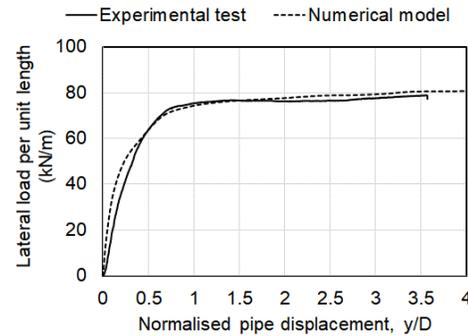
Figure 8. p-y responses of pipeline in numerical model and experimental test.
