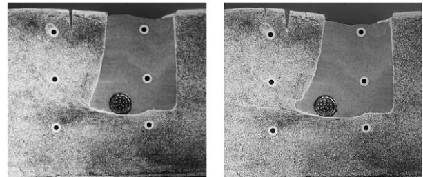
Figure 12. Crack shown in native ground
