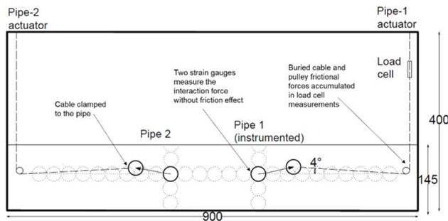
Figure 1. Schematic view of test 1; initial and post-test location of pipe; all dimensions are in mm
