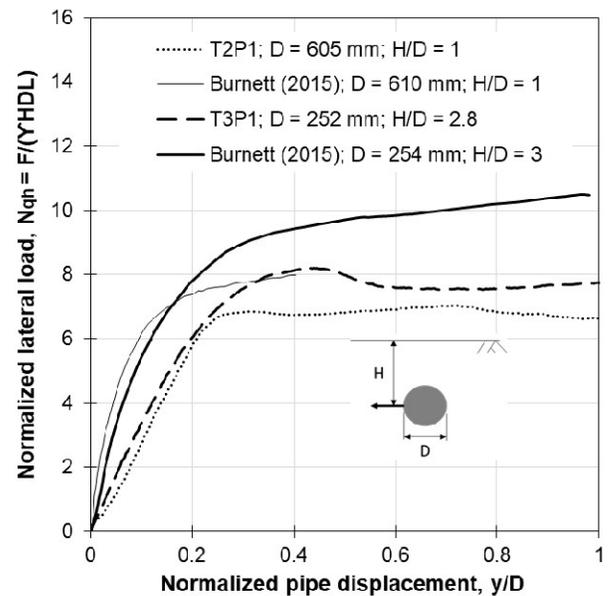
Figure 5. Comparison of the present study (very loose sand) with Burnett (2015) (full-scale loose sand)
