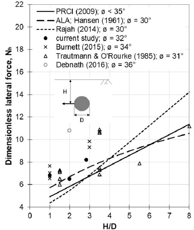
Figure 4. Comparison of the normalized resistance with several published test results and guidelines for loose sand
