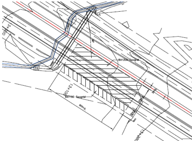
Figure 15 – Geogrid Placement at Station 13+100 EBL
