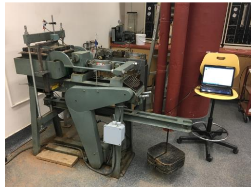
Figure 4. The large-scale direct shear box apparatus
