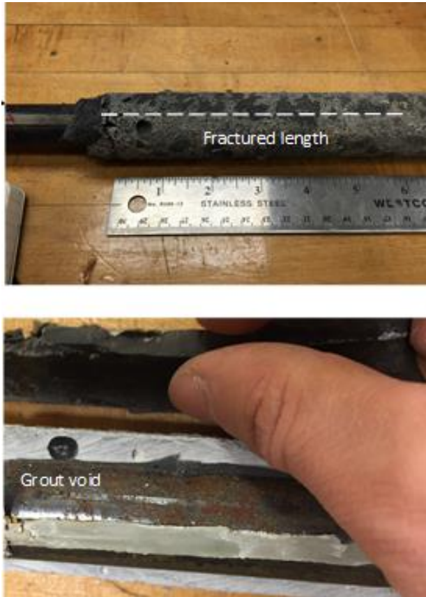
Figure 4. Axial Pullout Test. Post-test removal of the grouted length from the concrete block. (Top) Fracture extending 150 mm along the grout from the load end, aligned with the optical fiber; (Bottom) Void in the grout approximately 150 mm from the load end.
