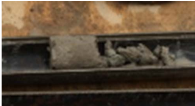
Figure 2. Photo of a hard till sample retrieval with a Split-Barrel Sampler (SPT).
