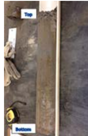
Figure 3. Photo of a till sample retrieved with Shelby Tube.
