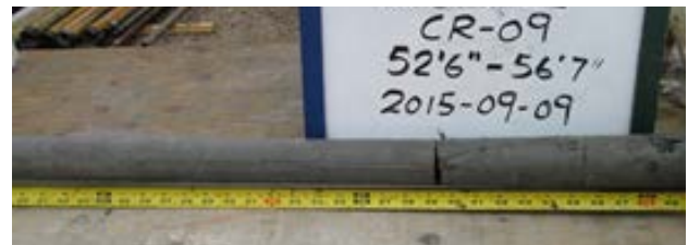
Figure 4. Photo of a till sample retrieval with core drilling.
