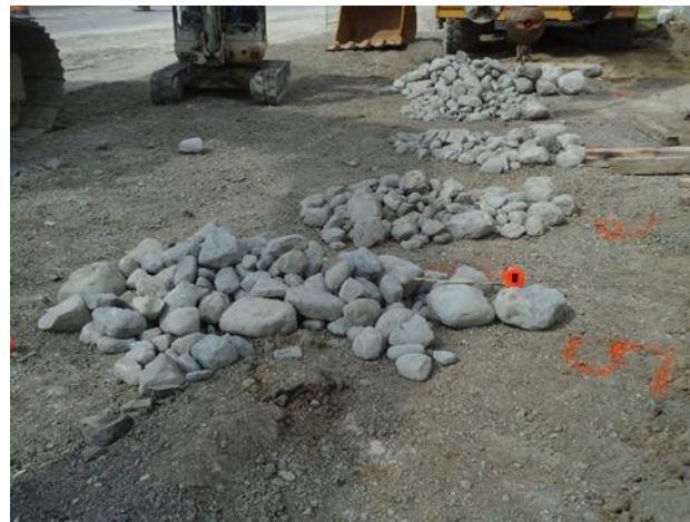
Figure 2. Segregation and depth-sorting of cobbles and boulders recovered from TBM rescue shaft, prior to sorting by size range
