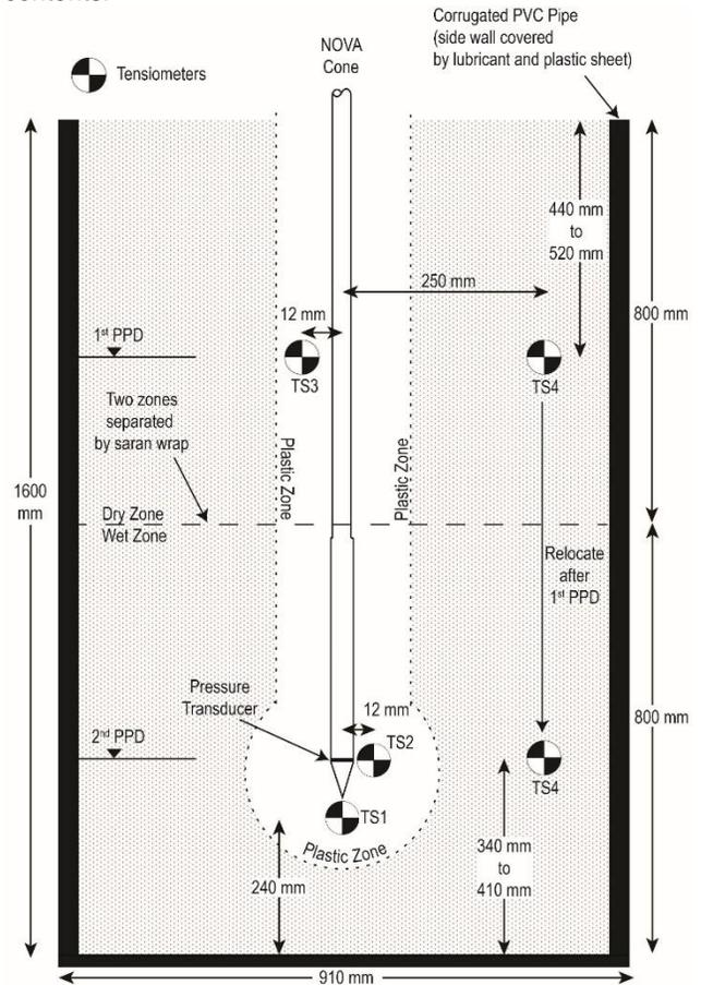
Figure 2: General Layout of Chamber testing
