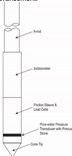
Figure 1: NOVA cone used for unsaturated soil testing
