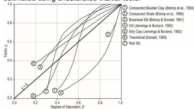
Figure 12: The  $\chi$  parameter against degree of saturation for various soils (After Jennings & Burland, 1962)
