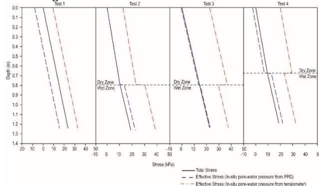
Figure 13: Calculated effective stresses for chamber tests
