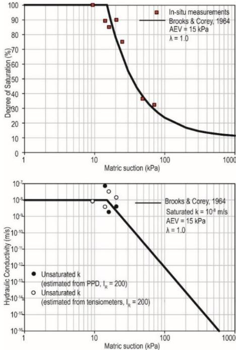
Figure 10: Estimated unsaturated hydraulic conductivity (In-situ condition)
