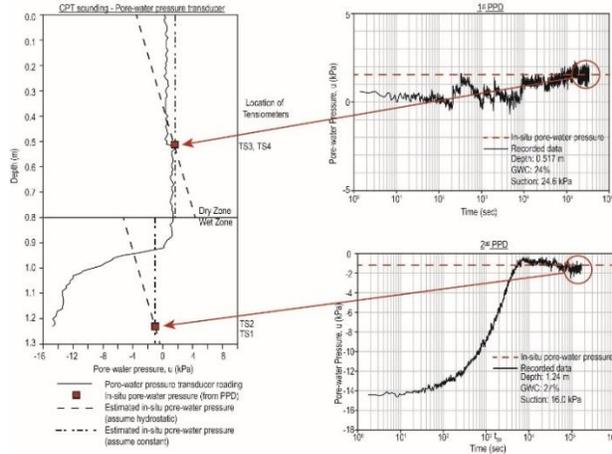
Figure 11: Interpreting in-situ pore-water pressure from PPD results
