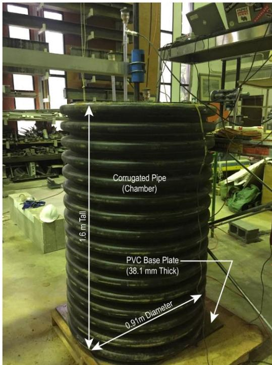
Figure 5: Photo of Chamber Test Set-up
