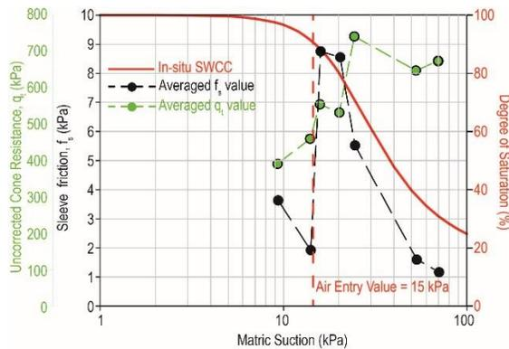
Figure 7: Matric suction against averaged sleeve friction & averaged corrected cone resistance
