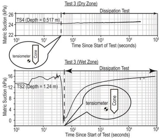
Figure 9: Two Types of Matric Suction Responses (Test 3)
