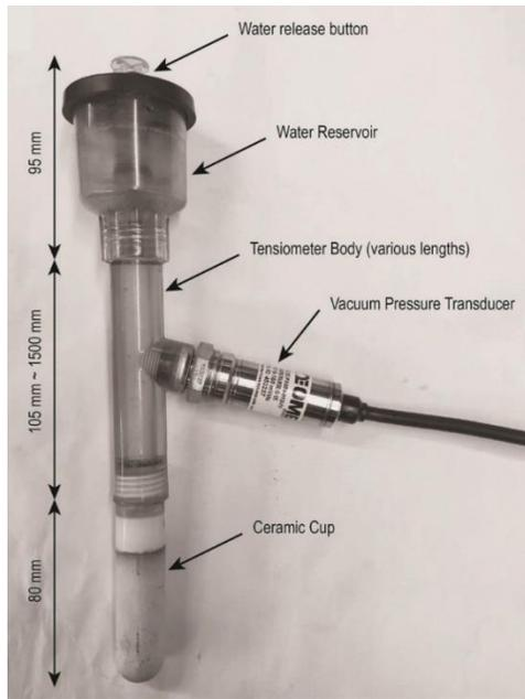
Figure 3: Jet-fill type tensiometer
