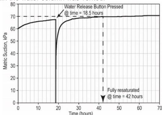
Figure 4: Re-saturation of tensiometer before Test 3
