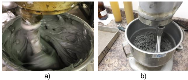
Figure 1. Consistency of material before (a) and after (b) the addition of quicklime and LKD
