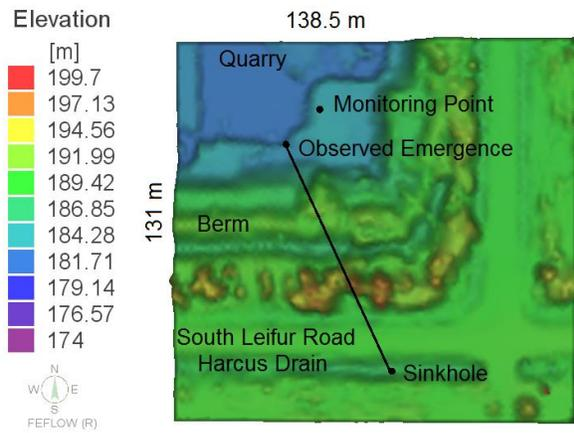
Figure 1. The study area. Inflow marks the location of the sinkhole and tracer injection, outflow the location of the fluorometer monitoring. Emergence is the point the tracer was first visible. The black line indicates the model location.
