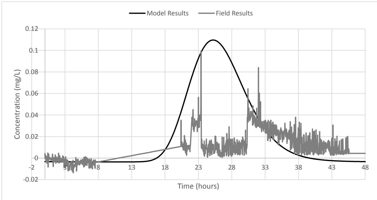
Figure 5. Comparison of observed breakthrough curve (grey) and modelled breakthrough curve (black for the tracer test, observed at the quarry). Hydraulic head difference of 0.5 m, fracture thickness 0.003 m, diffusion  $1 \times 10^{-5} \text{ m}^2/\text{s}$ , longitudinal dispersivity 1.2 m, transverse dispersivity 1 m.
