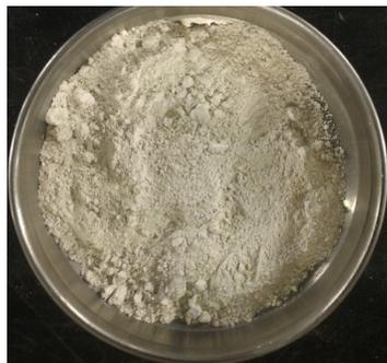
Figure 4. Hydrated lime used in this investigation
