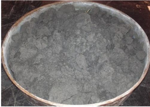
Figure 2. Sugar-cane bagasse ash
