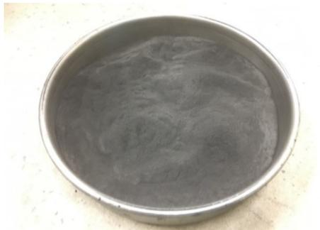
Figure 3. Selected sugar-cane bagasse ash employed in this study
