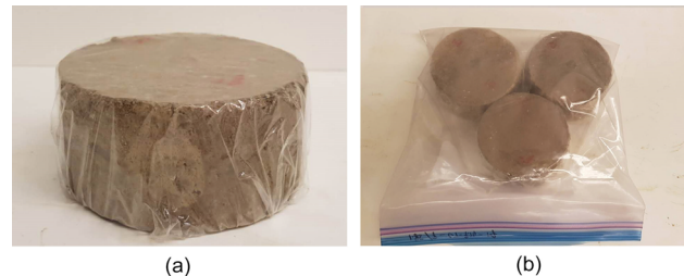
Figure 5. Standing specimens (a) wrapped by plastic film (b) sealed in zip-lock bag
