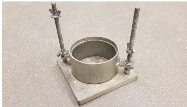
Figure 3. Compaction mold for the specimens
