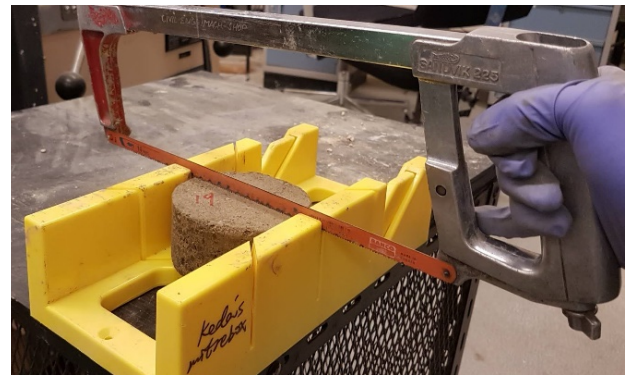
Figure 4. Sawing the specimen with hand saw guided by miter box
