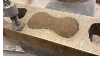
Figure 9. Compacted dog-bone specimen in the mold
