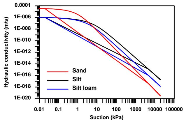
Figure 5. Hydraulic conductivity functions (model: Mualem 1976) (after Bashir et al. 2017)
