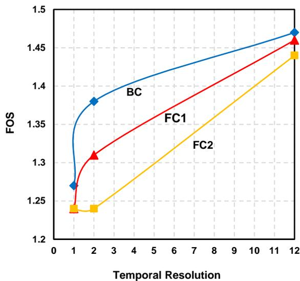
Figure 7. Variation of FOS of the sand embankment with temporal resolution of precipitation
