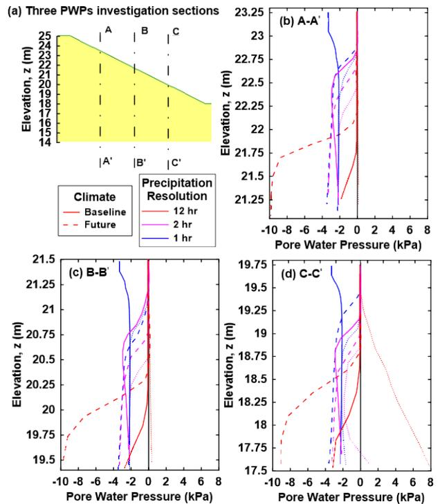
Figure 8 (a) Location of the three vertical sections, (b), (c), and (d) PWP distributions for the three climate ensembles and three temporal resolutions of precipitation at the A-A', B-B', and C-C' sections respectively
