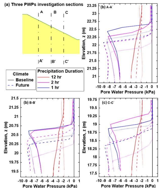
Figure 6. (a) Location of the three vertical sections, (b), (c), and (d) PWP distributions for three CEs, and three temporal resolutions of precipitation at the top, middle, and bottom sections of the sand embankment
