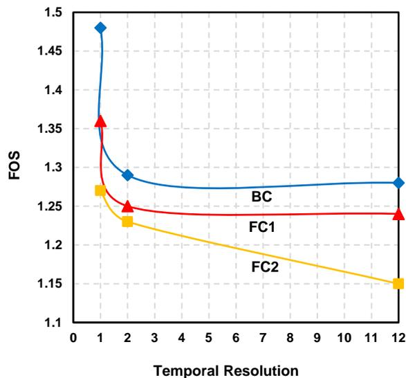
Figure 9. Variation of FOS of the silt embankment with temporal resolution of precipitation
