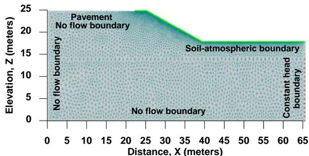
Figure 3. Design embankment profile with FEM mesh and boundary conditions
