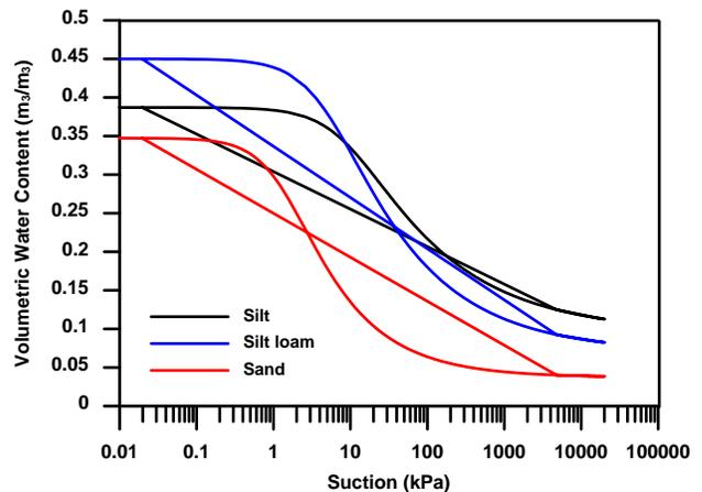
Figure 4. Soil water characteristic curves (model: van Genuchten 1980) (after Bashir et al. 2017)
