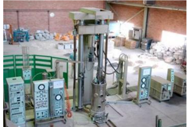
Figure 2. Large-diameter cyclic triaxial device in the Soil Dynamics Laboratory of BHRC
