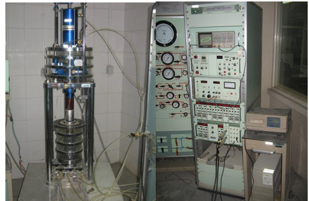
Figure 3. Regular size cyclic triaxial testing device equipped with resonant column testing facilities
