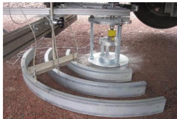
Figure 3. APLT test setup with deformation measurements obtained at 2r, 3r and 4r from the center axis. (White and Vennapusa, 2016)
