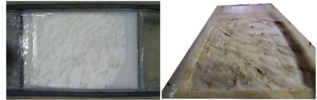
Figure 5. The sample before (left) and after (right) test 2 (flow rate of 0.33 m/s-pure gypsum)
