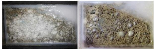
Figure 6. The sample before (left) and after (right) test 5 (flow rate of 0.33 m/s- gypsum plus other soluble materials)
