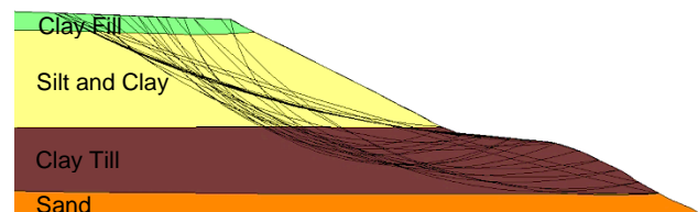
Figure 1. Typical model showing multiple slip surfaces, which all mathematically yield a FOS of 1.50
