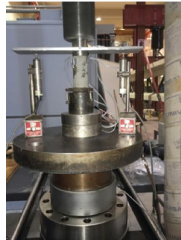
Figure 2. Setup for uniaxial compression test (2.2 MN load frame in the University of Calgary lab)
