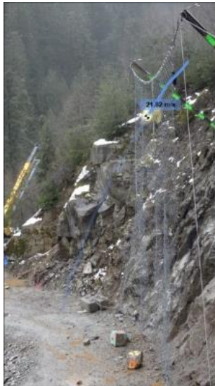
Figure 7: tracking of a block throughout its fall with the software Kinovea.
