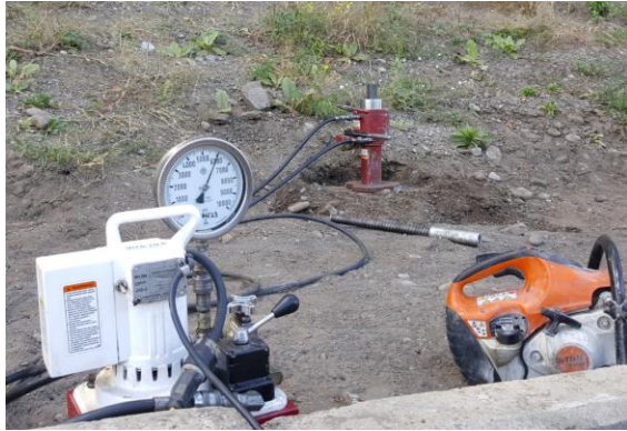
Figure 12. Confirming pull-out resistance with jack stand
