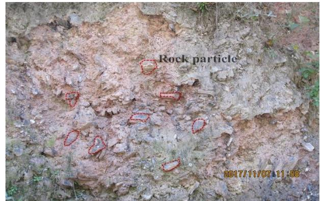
Figure 1. Soil and rock particles mixture of the sampling spot
