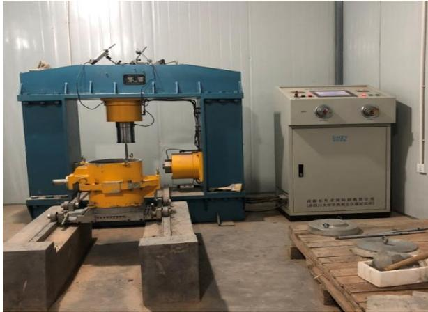
Figure 3. Photo of the large-scale direct shear test apparatus
