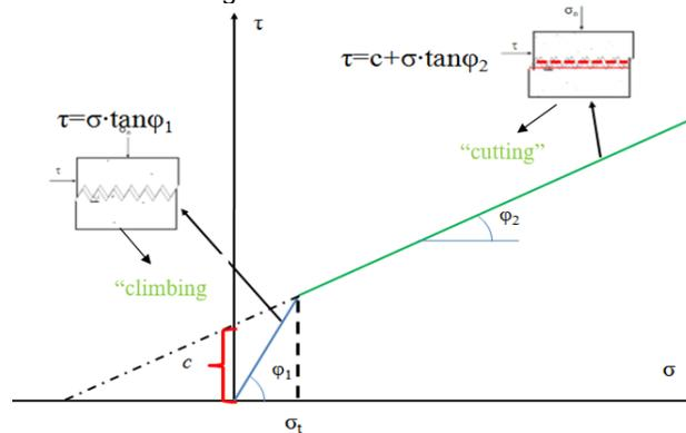
Figure 5. The bilinear strength criterion of PATTO
