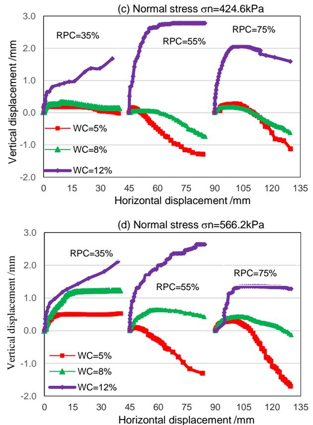
Figure 6. Vertical and horizontal displacement curves of the samples with different water and rock particle contents under the same normal stress.
