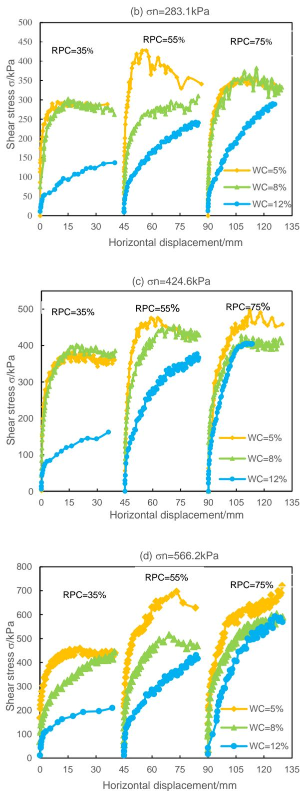
Figure 4. Shear stress and horizontal displacement curves of samples with different water and rock particle contents under the different normal stresses
