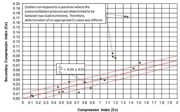
Figure 10. IL consolidation testing, relationship between secondary compression index ( $C_{\alpha}$ ) and compression index ( $C_c$ )
