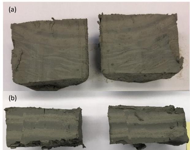
Figure 6. Silty and clayey layers/laminae observed on specimens recovered from (a) Borehole 1B Sample 10, and; (b) Borehole 3B Sample 6
