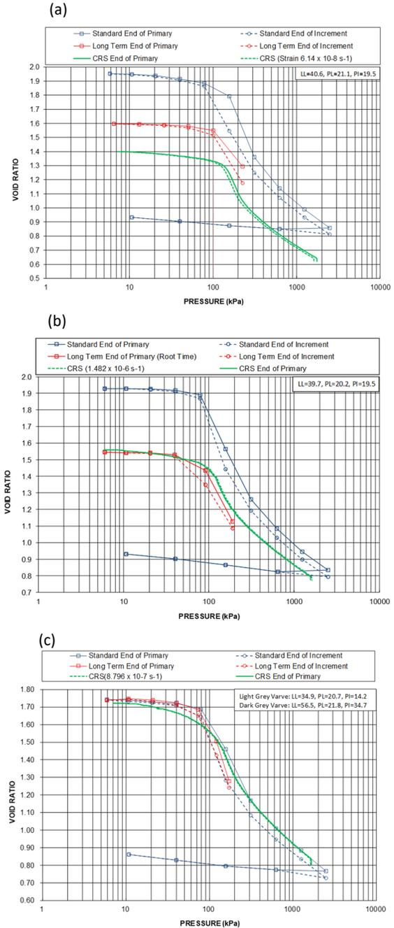
Figure 8. Comparison of CRS as well as standard and LT IL consolidation tests carried out on (a) Borehole 1B Sample 10; (b) Borehole 2B Sample 9, and; (c) Borehole 3B Sample 6
