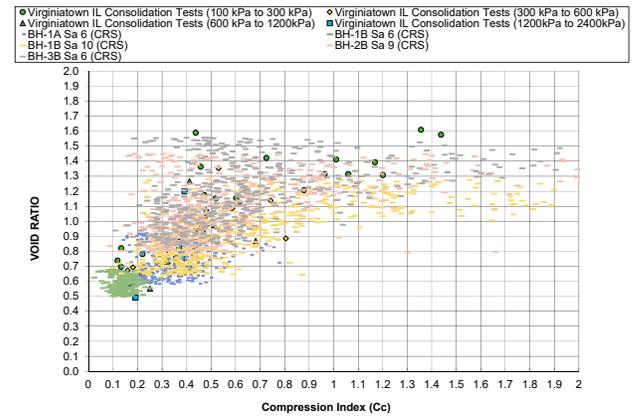
Figure 9. Consolidation testing results, relationship between void ratio and compression index ( $C_c$ )
