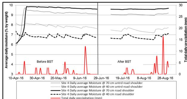
Figure 12. Comparison of precipitation and road moisture, site 4, spring and summer 2016
