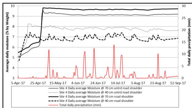
Figure 13. Comparison of precipitation and road moisture, site 4, spring and summer 2017
