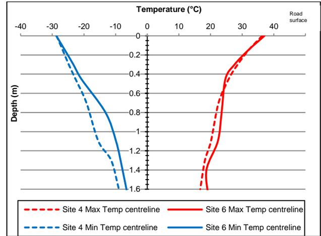
Figure 5. Centreline and shoulder temperature ranges with depth, sites 4 and 6 in, 2016 to 2018
