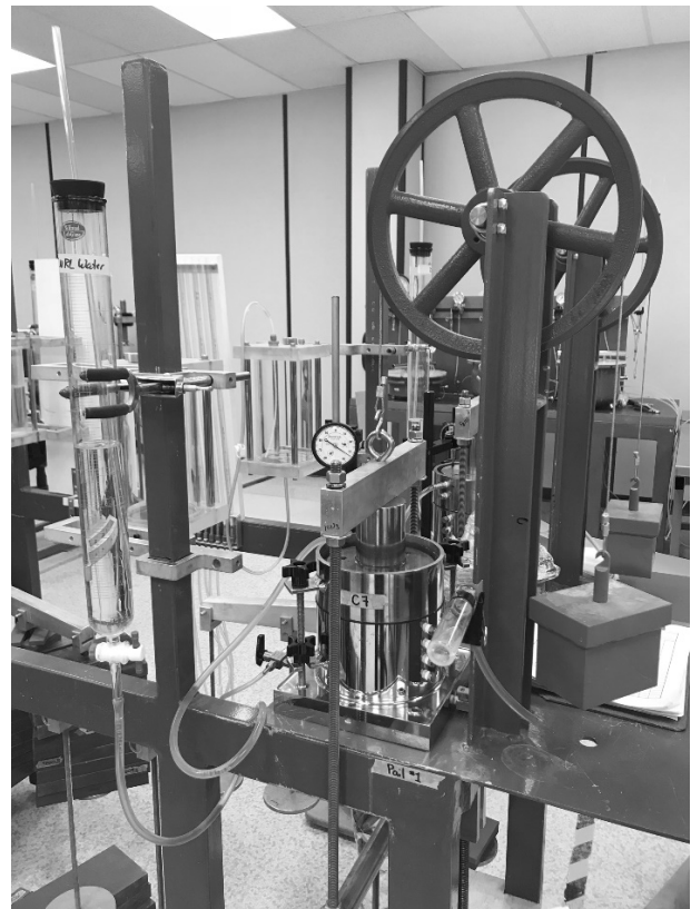
Figure 2: Large-strain consolidation test apparatus
