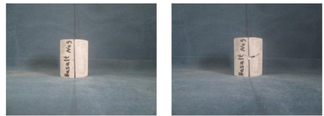
Figure 2. Rock core specimen obtained from ballast parent rock before and after diametral PLT
