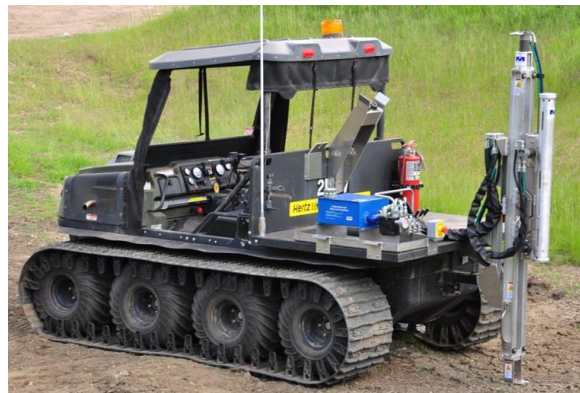
Figure 16. Automated Dynamic Cone Penetration rig
