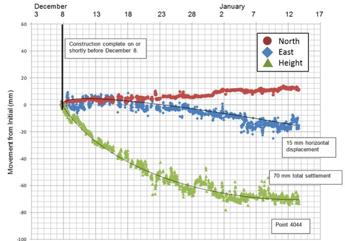
Figure 7. Pad settlement data from a 5 m lift
