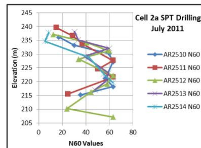
Figure 8. SPT results from 5 boreholes in the pad fill
