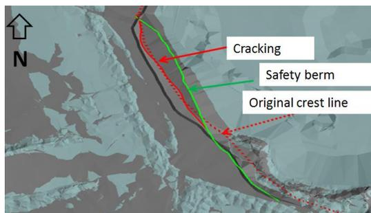
Figure 14. Slumping during Phase 2 backfill, showing safety berm (crest) location and slumping behind crest
