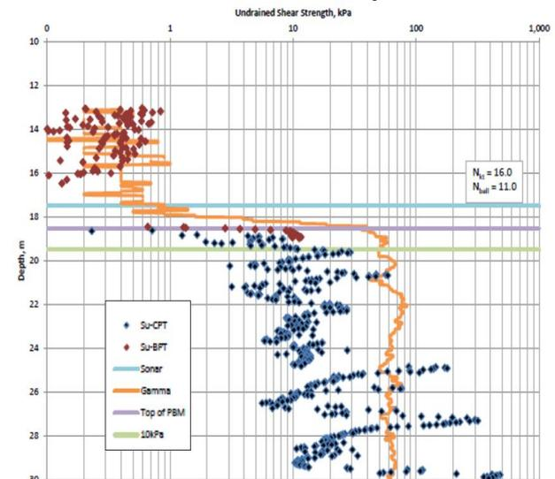
Figure 10. Typical BPT and CPT profile showing transition from mudline to solid PBM
