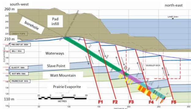
Figure 2. Schematic section through inflow location showing angled borehole and fault blocks (F1-F5)
