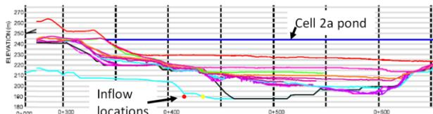
Figure 9. Multiple sonar profiles showing material flow across pond bottom during Phase 1 infilling, representing conditions at the start of Phase 2 infilling. Uppermost (red) line is June 2012 sonar.
