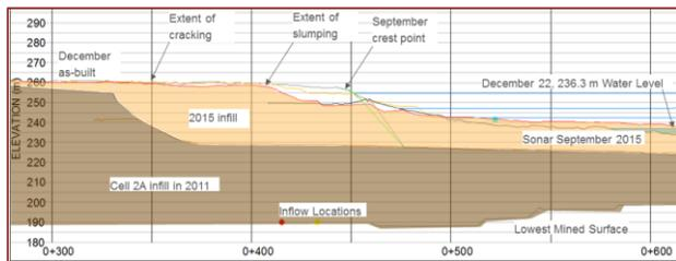
Figure 18. Progression of water drawdown and slumping
