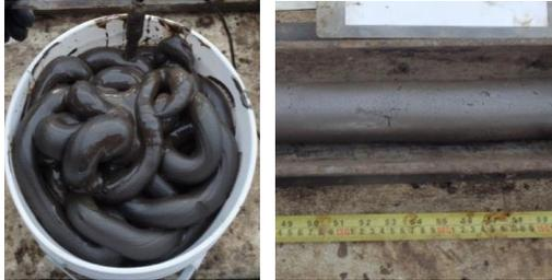
Figure 12: Transition from slurry to PBM (2 to 3 m below mudline) and PBM (7 m below mudline)
