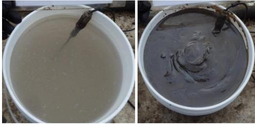
Figure 11: Saline Water (1 m above mudline) and slurry (1 to 2 m below mudline)
