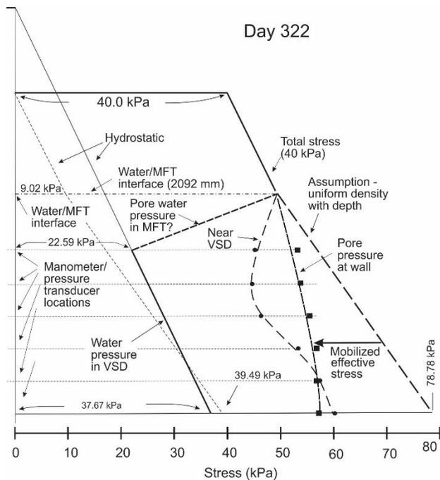
Figure 5: Stress distributions after 322 days of testing
