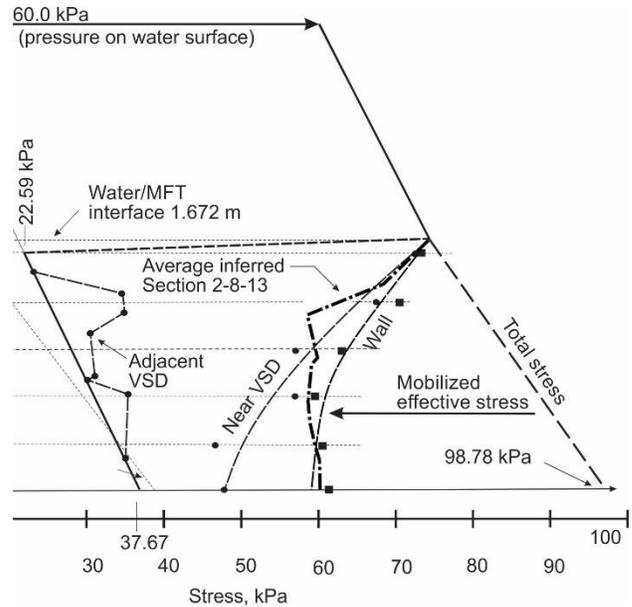
Figure 12: Comparison of monitoring and post-test sampling results.
