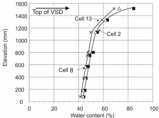
Figure 11: Post-test variation in water content with depth (elevation)
