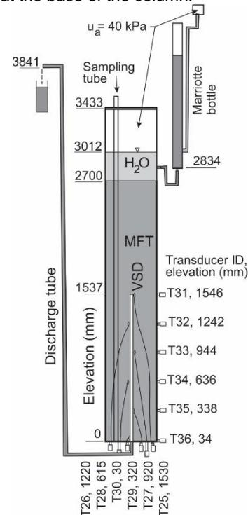
Figure 1: MFT test column design
