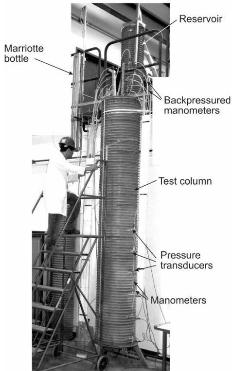
Figure 3: Test column in operation
