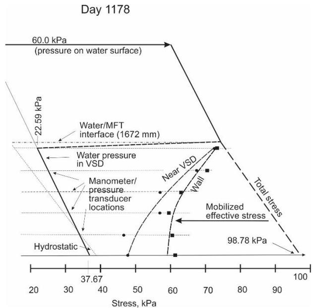
Figure 6: Stress distributions after 1178 days of testing
