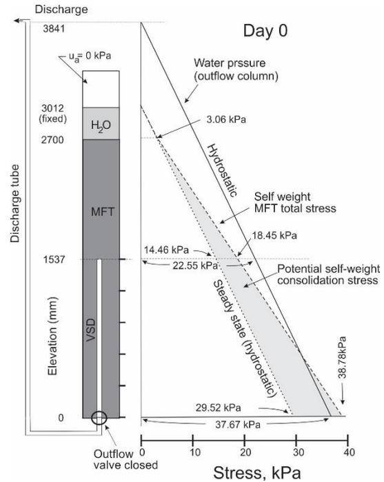
Figure 2: Stress distributions in the test column at Day 0, prior to testing.
