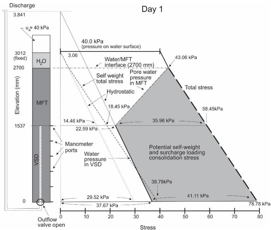
Figure 4: Stress distributions within the test column and outflow column
