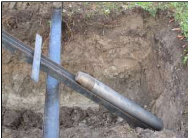
Figure 2. Shelby tube samples with inclined orientation
