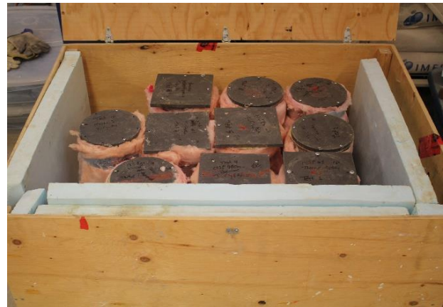
Figure 3. Each test consisted of a PVC column wrapped with glass fibre insulation (top) and placed in an insulated wooden box (bottom). (Photo: M. Hosney, Queen's University)
