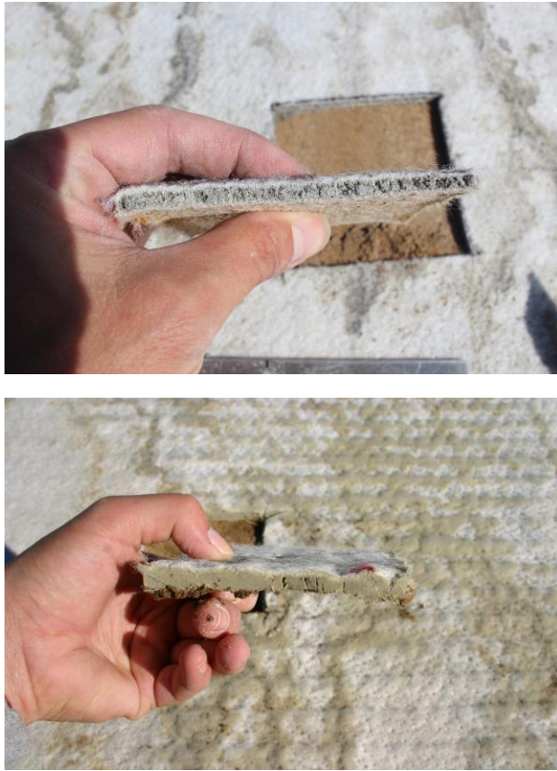
Figure 1. Photographs of GCL 2 (top) and GCL 6 (bottom) specimens cut from GCL panels at QUELTS after 3.5 months of field exposure when covered only by a black geomembrane. For scale, the specimens are 100 mm x 100 mm.
