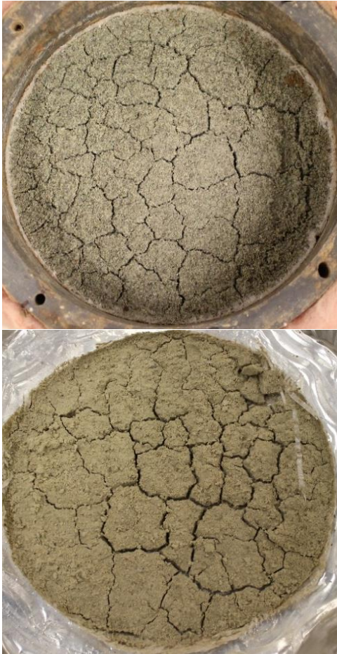
Figure 7. Desiccation cracks observed in GCL 2 (top) and GCL 6 (bottom) deconstructed specimens after seven daily thermal cycles.
