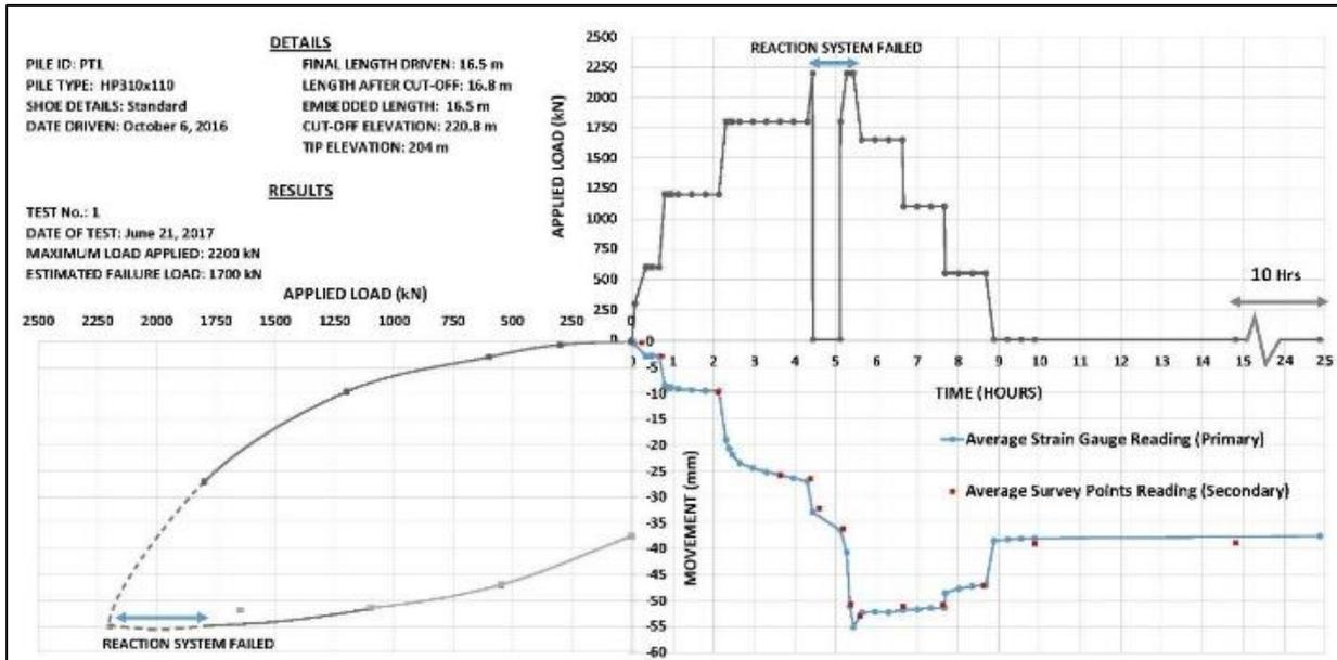
Figure 4b: Static pile load test results - Site #2
