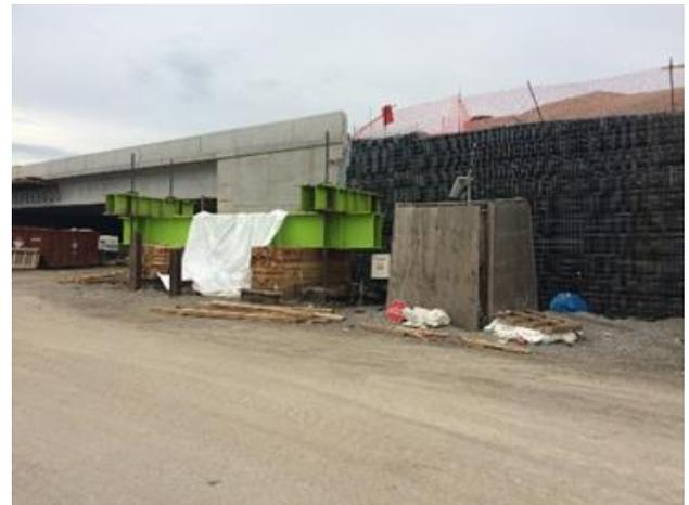
Figure 3b - Site #2 Pile Load Test Set-Up
