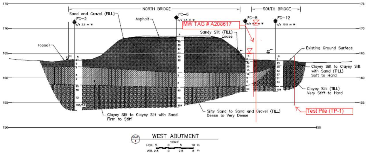
Figure 1a: Site #1 - Typical subsurface section at the area of the test pile
