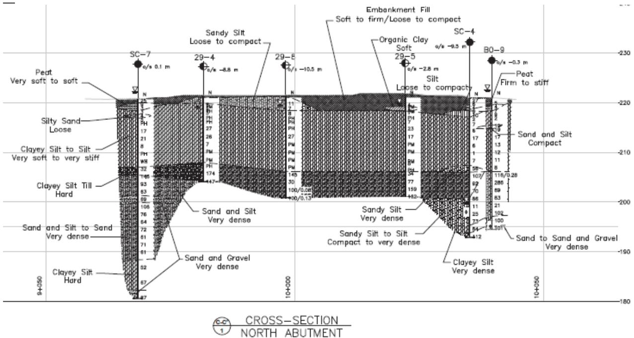
Figure 1b: Site #2 – Typical subsurface section at the area of the test pile
