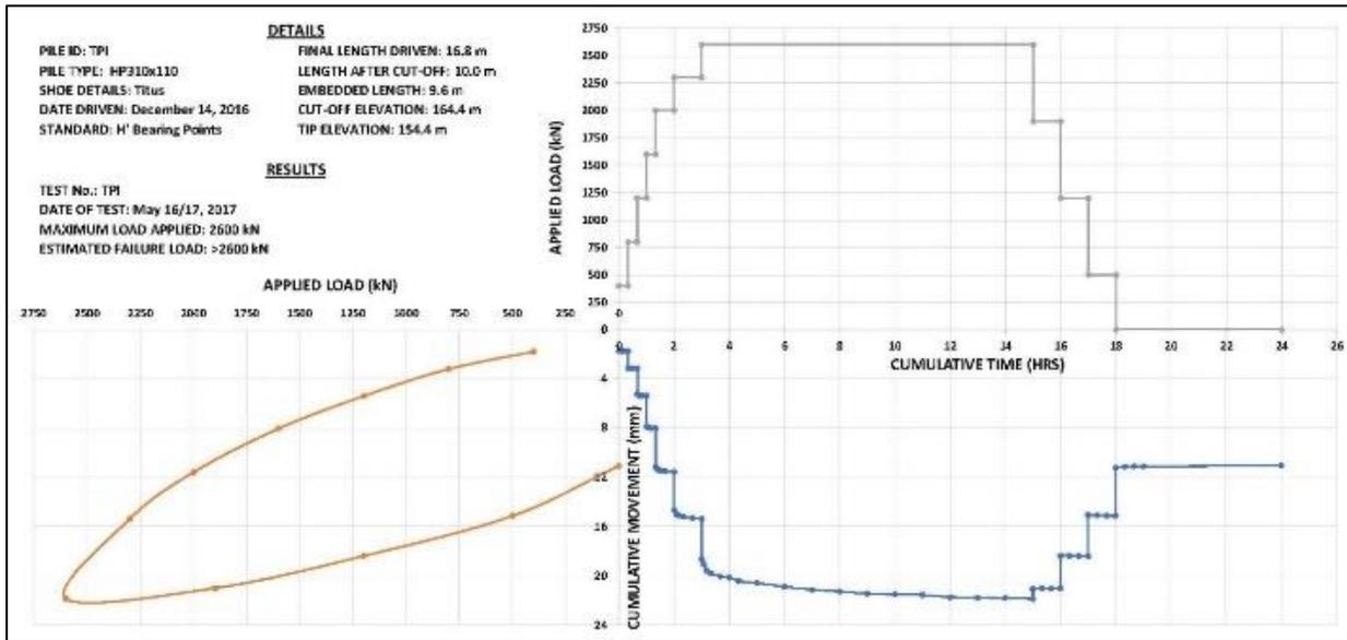
Figure 4a: Static pile load test results - Site #1
