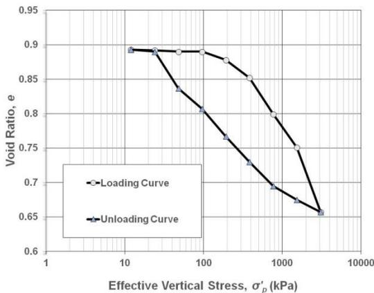
Figure 6. 1-D consolidation test results of upper Lea Park Shale from beneath the North Saskatchewan River bed. (Clifton Associates, 1983)
