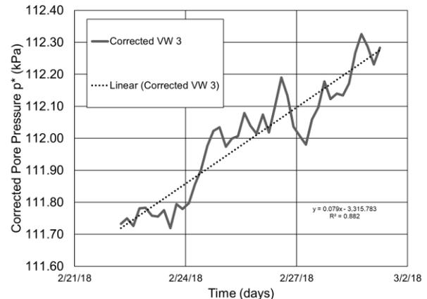
Figure 4. BH501 corrected pore pressure vs. time. Determining loading efficiency visually while correcting for barometric loading in Lea Park Shale
