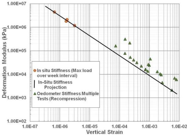
Figure 7. Relationship of deformation modulus with respect to vertical strain increment
