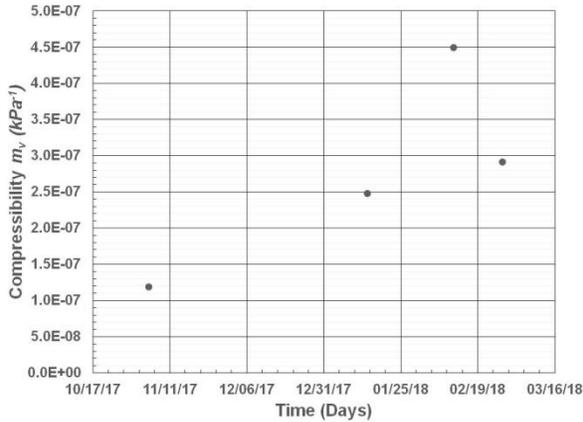
Figure 5. Change in In-situ compressibility  $m_v$  due to barometric loading over the time of monitoring
