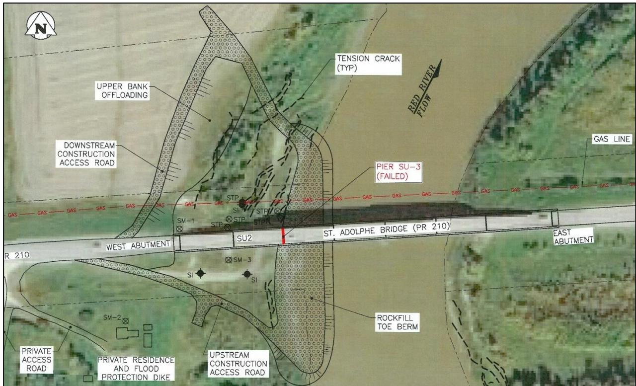
Figure 9. Plan of emergency stabilization works.
