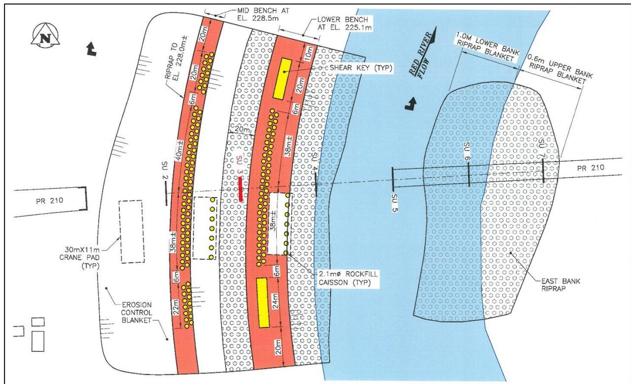
Figure 15. Plan of permanent stabilization works.
