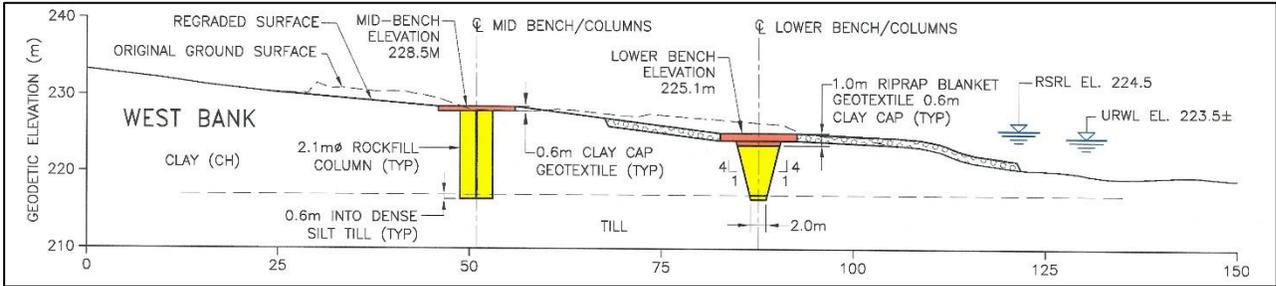
Figure 14. Section of permanent stabilization works.
