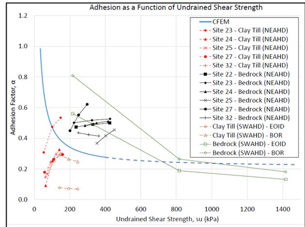
Figure 9. “Adhesion factor as a function of undrained shear strength” from CFEM (2006) including NEAHD and SWAHD data
