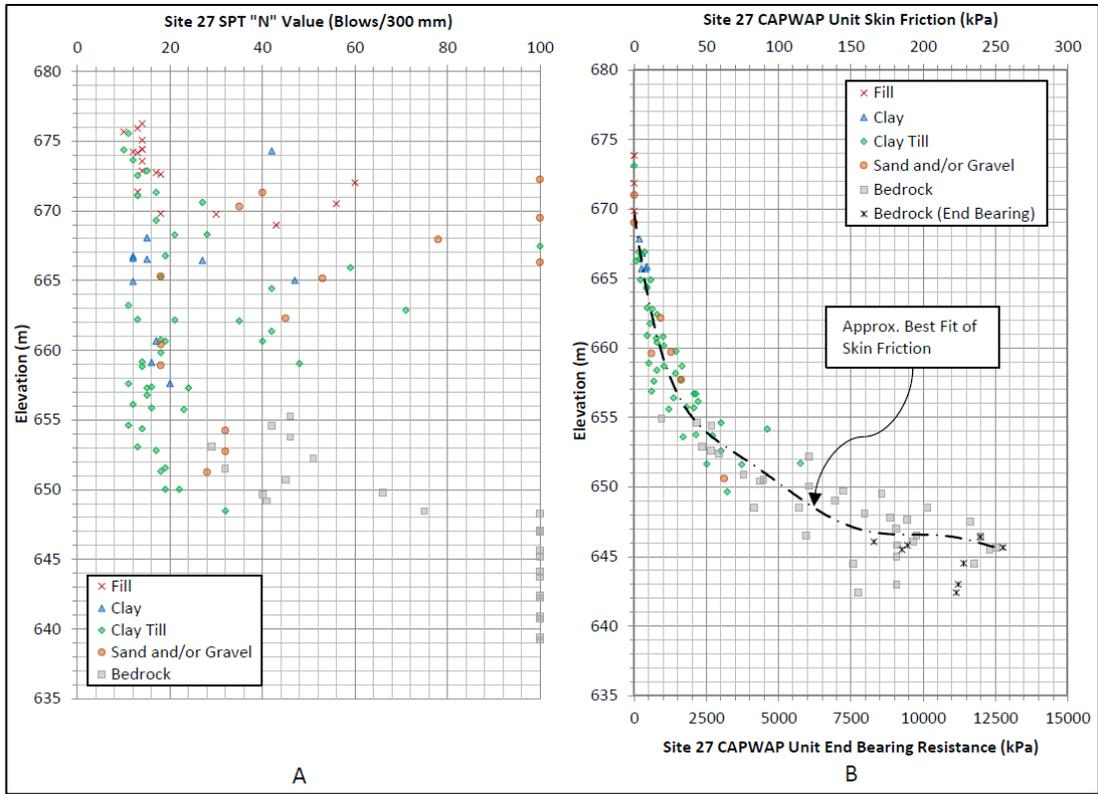
Figure 7. A) Site 27 variation of SPT 'N' values with elevation
