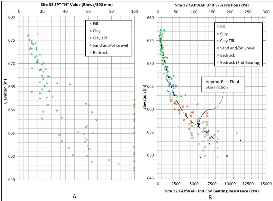
Figure 8. A) Site 32 variation of SPT 'N' values with elevation
