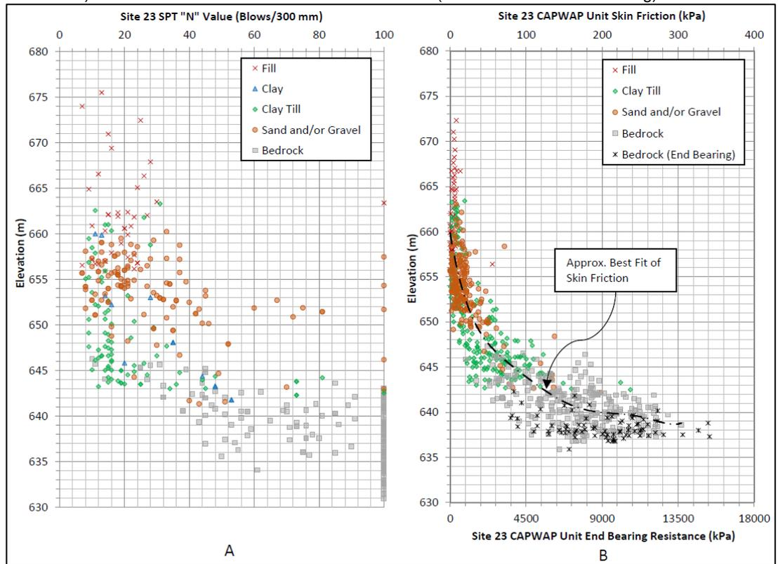
Figure 4. A) Site 23 variation of SPT 'N' values with elevation
