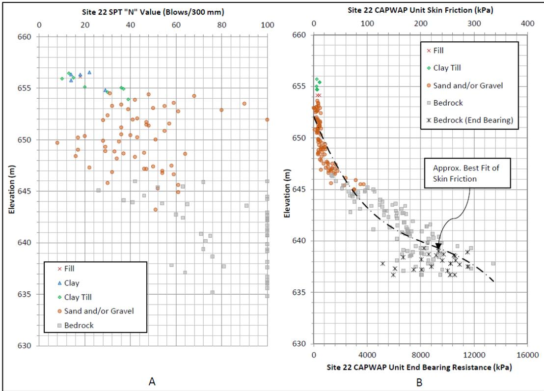
Figure 3. A) Site 22 variation of SPT 'N' values with elevation
