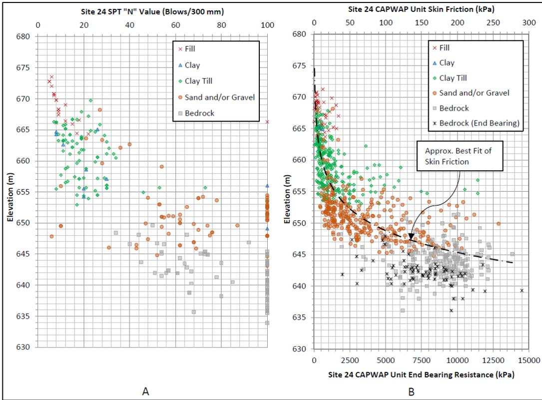
Figure 5. A) Site 24 variation of SPT 'N' values with elevation
