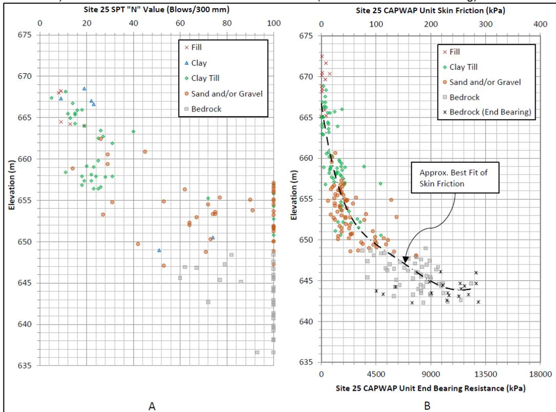
Figure 6. A) Site 25 variation of SPT 'N' values with elevation
