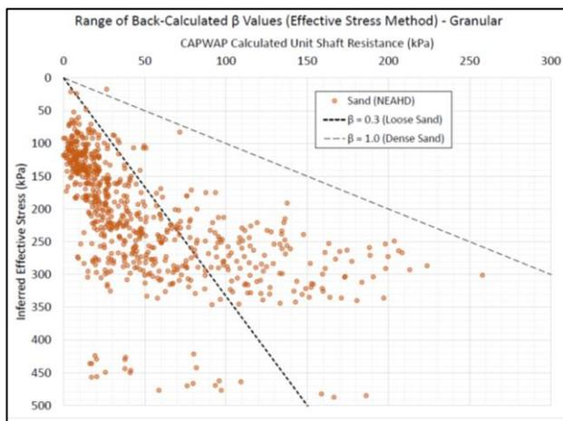
Figure 11. Back-calculated combined shaft resistance factors for granular soils from NEAHD data
