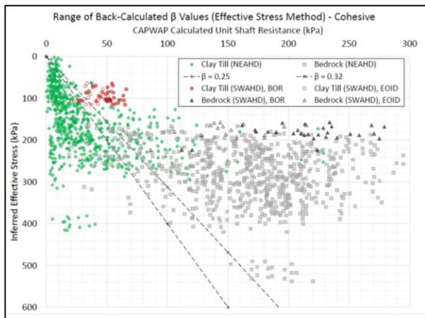
Figure 10. Back-calculated combined shaft resistance factors for cohesive soils from NEAHD and SWAHD data
