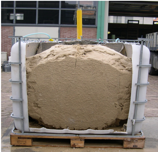
Figure 3. The cubic meter bio-grout experiment performed by van Paassen(2009) (picture shared by van Paassen Leon).
