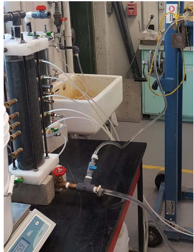
Figure 3. Experiment with a 60-L Mariotte bottle (not shown) as the constant-head reservoir. An electronic scale measures the water leaving the column. Tracers are injected through a septum in the T connection.
