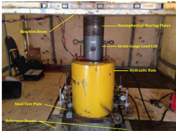
Figure 8: Compressive pile load test setup
