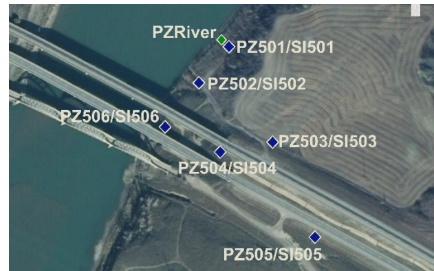
Figure 3. Layout of recent piezometers on east abutment
