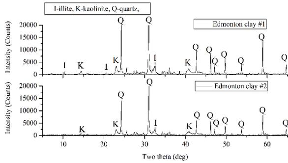
Figure 2: XRD test results of EC#1 and EC#2
