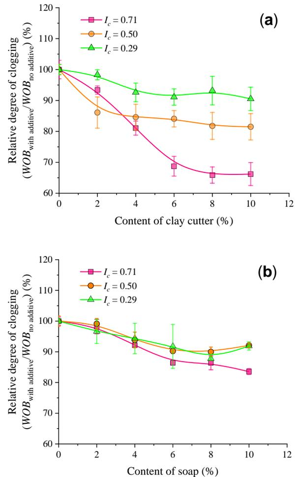
Figure 5:  $RDC$  for conditioned soils for (a) clay cutter and (b) soap
