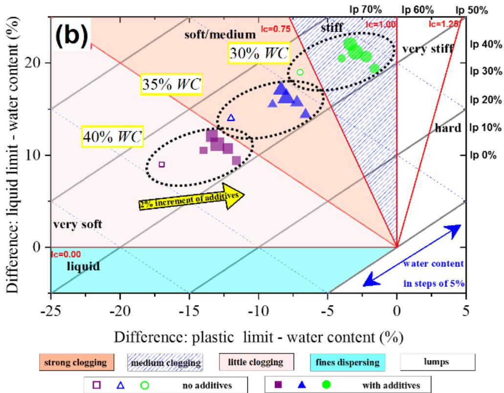
Figure 6: Performance of soil additives evaluated using semi-empirical diagram (a) clay cutter and (b) soap
