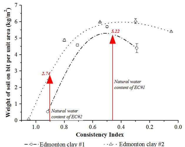
Figure 3: Clogging test results for different plain soils with natural water content labeled
