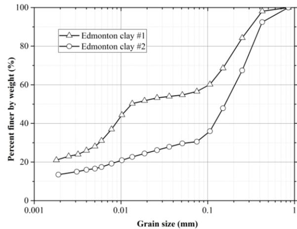
Figure 1: Particle size distribution curve for EC #1 and EC #2
