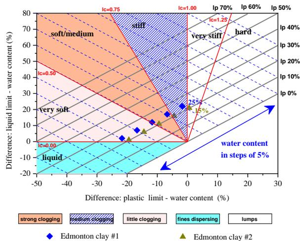
Figure 4: Plot of clogging results tested using the new apparatus on a universal diagram proposed by Hollmann & Thewes (2013)
