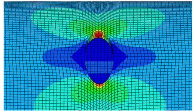
Figure 12. Maximum principal stress around an elliptical pit
