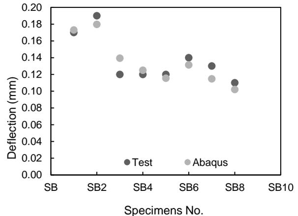
Figure 6. Comparison of deflection from test and Abaqus
