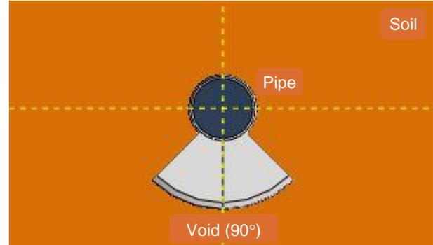
Figure 8. Symmetric void (90°) with respect to pit hole
