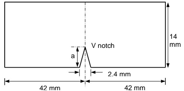
Figure 2. Test specimen used
