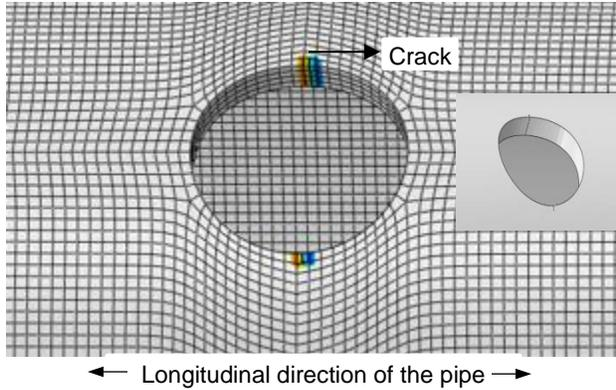
Figure 9. Crack propagation direction (phlism)
