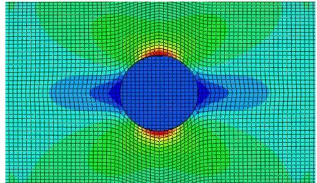
Figure 11. Maximum principal stress around a circular pit
