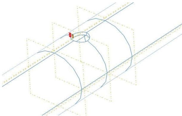
Figure 7. Crack extension direction in Contour integral method
