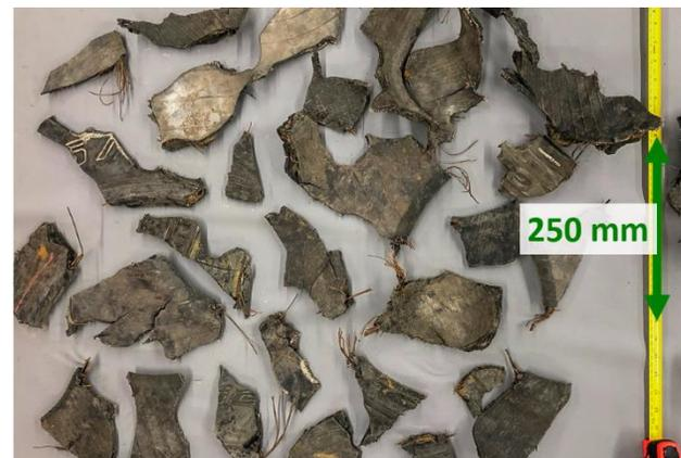
Figure 13: High risk TDA pieces containing isolated small diameter wires
