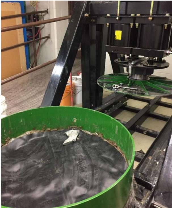
Figure 1: Large pneumatic simulated landfill loading testing device
