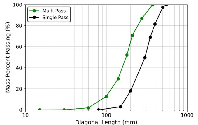
Figure 2: Grain size distribution of TDA used in testing
