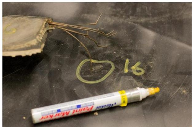
Figure 8: Puncture from test 3
