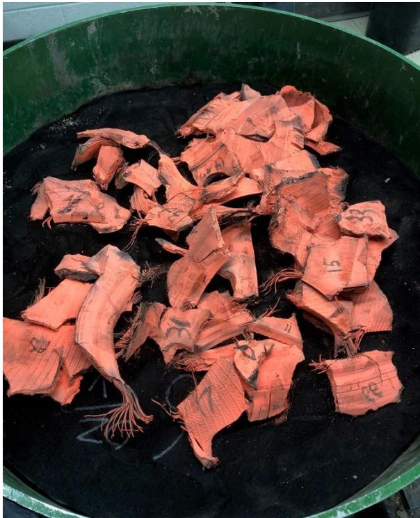
Figure 3: Pre-sorted TDA pieces from Sample 1 with unfavorable protruding wires placed intentionally on geotextile
