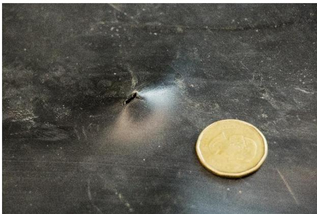
Figure 5: Puncture from test 1 (bottom view)
