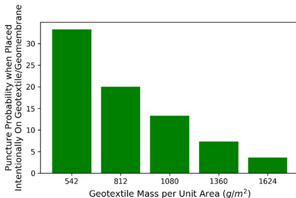
Figure 11: Probability of puncture given that the TDA piece falls in an unfavourable position
