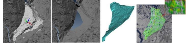
Figure 6: Analysis of a fallen block, showing from left to right: Surface of block prior to failure, back fracture following failure, visualization of the detached shape from behind and analysis of the roughness of the sliding surface. (after Graham et al, 2018).
