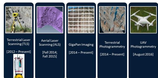
Figure 1: Remote sensing techniques used for rock slope stability analysis in the RGHPR project.
