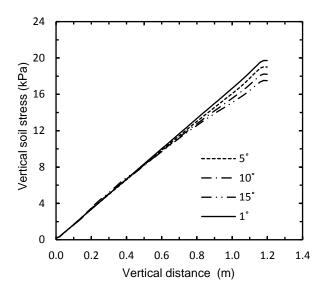
Figure 4. Vertical stresses with soil depth, 0.2 m away from the cell wall (initial loading).
