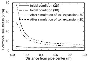
Figure 8. Horizontal soil stresses at springline level from pipe centre to cell wall.
