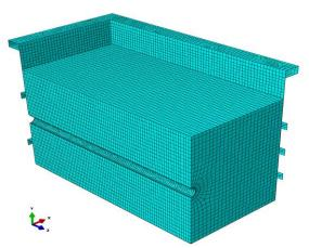
Figure 3. Typical finite-element mesh of soil, test cell and pipe used in 3-D model
