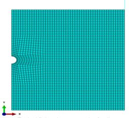
Figure 2. Typical finite-element mesh of soil, test cell and pipe used in 2-D model
