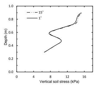
Figure 5. Vertical stresses with soil depth, 0.2 m away from the pipe centre during expansion.
