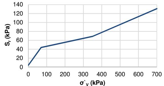
Figure 6. Post-liquefaction undrained shear strength.
