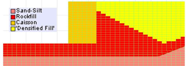
Figure 9. FLAC mesh near caisson showing relative grid spacing (note: background grid at units of 10 m).
