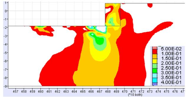
Figure 10. Initial shear stress and static shear stress ratio ( $\alpha$ ) at end of static analysis.
