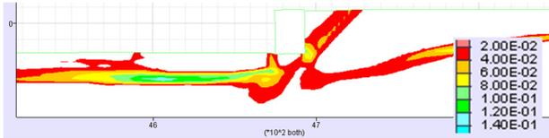
Figure 13. Estimated shear strain ( $\gamma_{xy}$ ) for 975-year Hector Mine motion. Multiply legend by 200 to convert  $\gamma$  in %.
