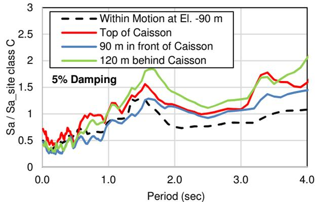
Figure 17. Response spectra amplification ratios for selected acceleration histories for 975-year Hector Mine motion.
