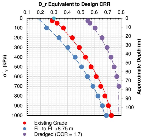
Figure 7. Selected profiles of  $D_r$  for calibrated model.
