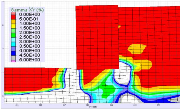
Figure 14. Estimated shear strain ( $\gamma_{xy}$  in percent) in vicinity of caisson for 975-year Hector Mine motion (end of earthquake). (note: white contours indicate shear strains in excess of 5%).
