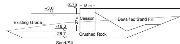
Figure 2. Caisson wharf section used for FLAC analysis
