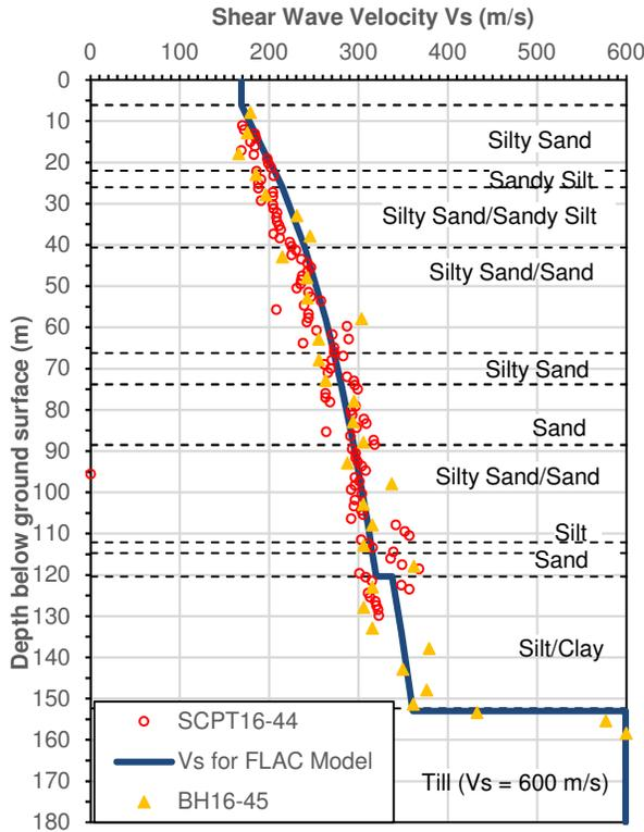
Figure 4.  $V_s$  measurement for selected soundings and  $V_s$  profile adopted for FLAC model.
