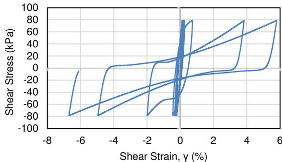
Figure 8. Shear stress – shear strain behavior from a single element FLAC simulation for a select stress state.
