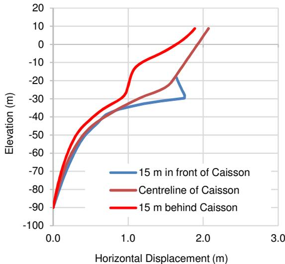
Figure 14 Horizontal displacement profiles at selected points for updated 975-year Hector Mine motion (end of earthquake).
