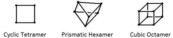
Figure 2. Condensed silicate anion structures. Dots represent silicon atoms and lines oxygen atoms.
