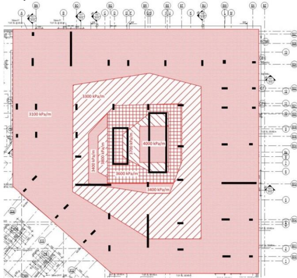
Figure 3. Calculated Subgrade Reaction Values at SLS
